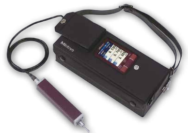
Transverse tracing drive unit Best suited for measurement of narrow, shrouded workpiece features such as crankshaft, EDM parts, etc.
