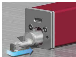
Retractable drive unit The detector is in the retracted position at rest so it is immune from damage when inserted into a feature whose profile cannot be easily seen, such as a blind hole, etc.
